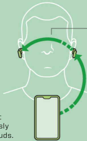
Bluetooth signal is relayed directly from the primary bud to the other bud. Bluetooth signal is sent to a single earbud.
